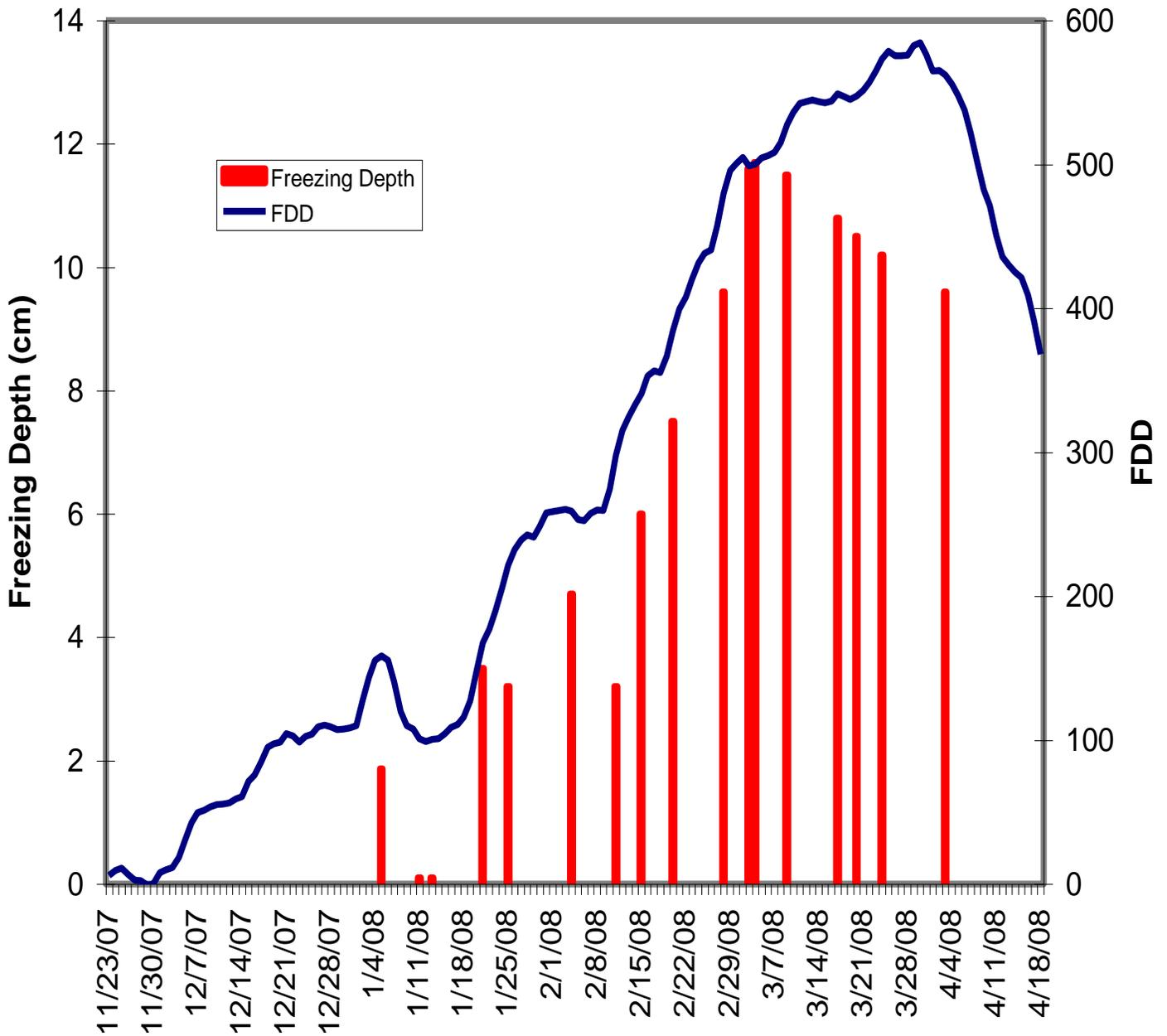
Figure 3. Accumulated FDD's and soil freezing depths.
