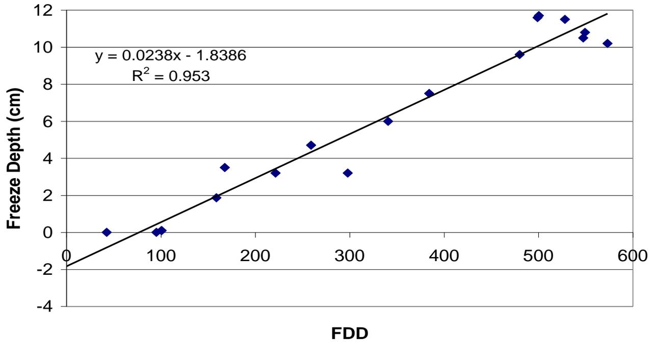
Figure 4. Correlation between FDDs and soil freezing depth.
