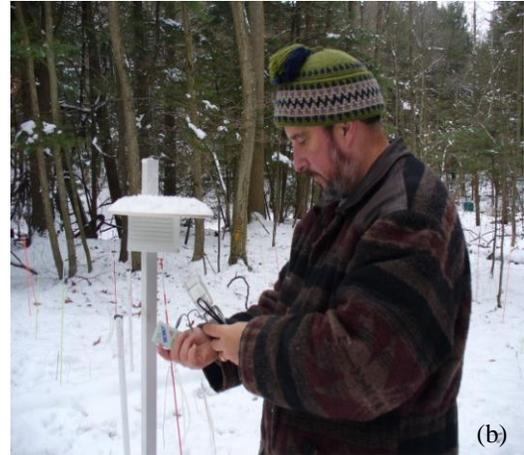
Figure 2. Frost tube inserted into a PVC pipe (a). Uploading air temperature from the data logger (b). The temperature data logger protective housing is shown.
