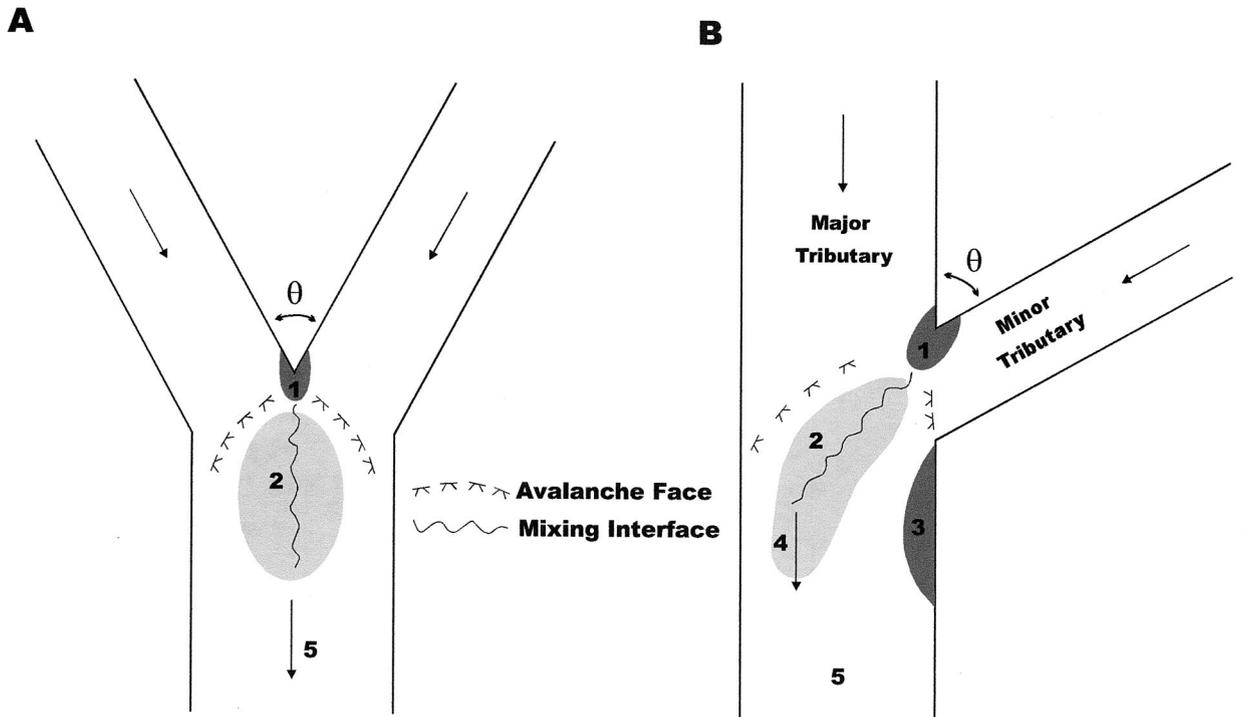
**Figure 4.** Characteristic assemblage of hydrodynamic/bar elements at symmetrical (A) and asymmetrical (B) confluences. Major elements include: (1) flow stagnation and stagnation-zone bar, (2) flow deflection and scour hole, (3) lateral flow separation and separation-zone bar, (4) maximum velocity and scour extension, and (5) zone of flow recovery and transverse bar (after Best 1987).
