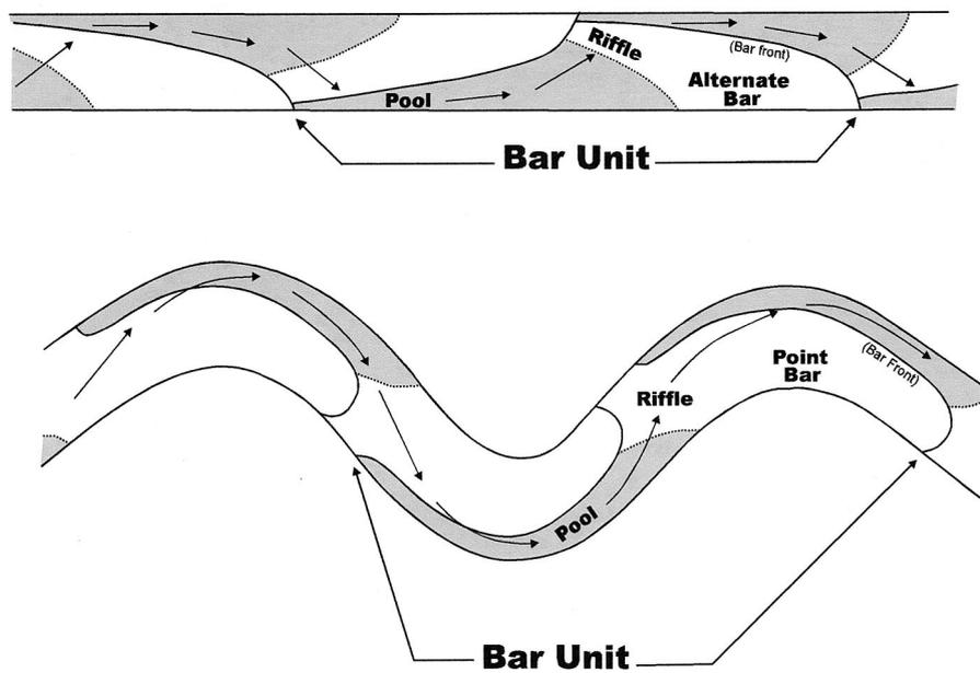
**Figure 3.** Plan view of bar units in straight (top) and meandering (bottom) channels. Shaded areas correspond to portions of the bed below the mean bed elevation. The highest elevation occurs at the portion of the bar unit corresponding to the alternate bar or point bar. Path of thalweg (thread of highest velocity) is indicated by arrows (after Dietrich 1987).
