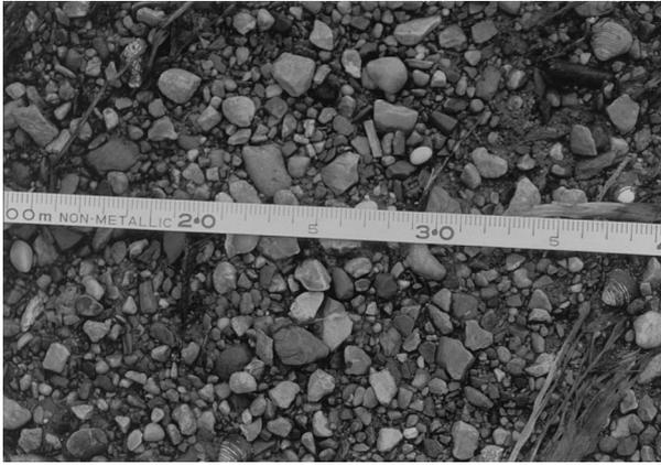
**Figure 5.** Fine gravel armor layer at the head of a point bar in the Kaskaskia River, East Central Illinois. Numbers on tape are tenths of a meter.
