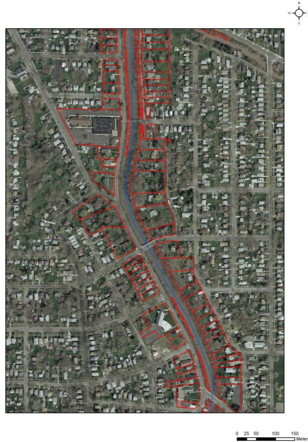
Figure 2. Map of the 46 m (150 ft) buffer and resultant parcels (outlined in red) in a representative section of Cayuga Creek.
